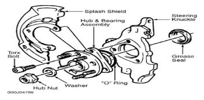
Fig. 3: Exploded View Of Hub & Bearing Assembly Courtesy of GENERAL MOTORS CORP.
