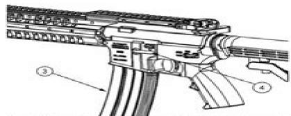
Insert loaded magazine (3) into rifle's magazine well until magazine catch (4) engages and holds cartridge magazine. Tap upward to make sure cartridge magazine is seated correctly.
