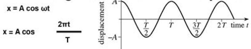
Timing from equilibrium gives a sine equation. Both are sinusoidal.
