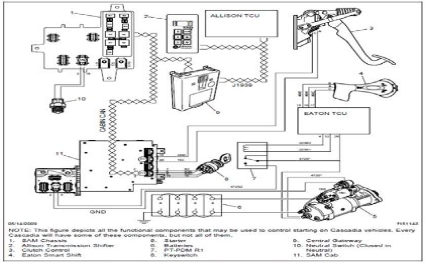
Fig. 2, Cascadia Starting Circuit, Without Optimized Idle Option
