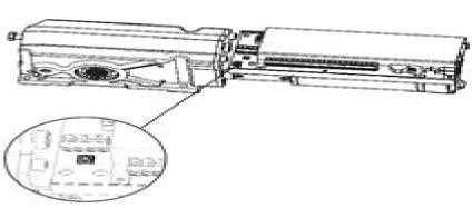
After completion of the mechanical installation and prior to adjusting the parameters, always initiate a calibration run by pressing and holding the pushbutton for 3 flashes of the red LED. This will insure proper door operation by calibrating the unit to the installation conditions.
