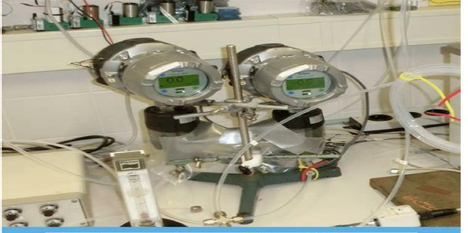
Laboratory tests of Draeger Polytron 8000 with FL- 6813260 sensor for NH3 measurement
