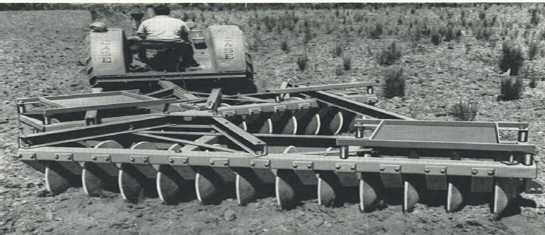
24-PLATE LITTLE GIANT WORKING FALLOW IN VICTORIA. 9 FEET CUT.
