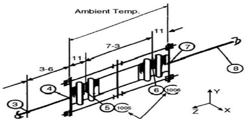
Zero length expansion joints with axial, lateral and torsional stiffnesses rigid, and no pressure thrust.
