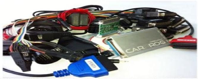
CARPROG was designed with regard to demands of our customers to have universal tool for car radios, odometers, dashboards, immobilizers repair including advanced functions like EEPROM and microcontroller programmer, key transponder programmer.
