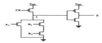
(b). When the clock signal changes from high to low and A, B, and B, are low, node I is charged from 0 to 2.5V through the pMOS transistor.
