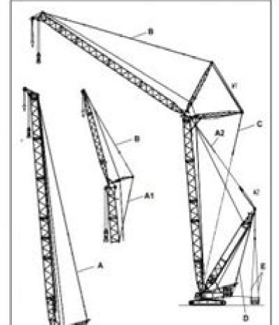
11.7 Chacking the Stay Bars, Bracing Rods and Mounting
