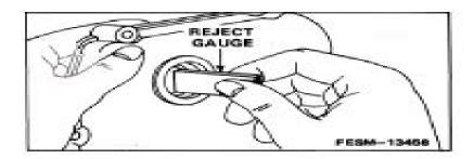
If 19166 or 19178 main bearing bore reject gauge will enter bearing, the bearing is worn excessively. Try the gauge at several locations.
