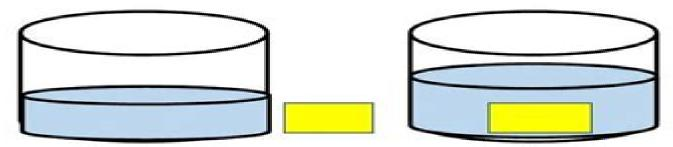
Volume of liquid without the submerged solid object = 200 ml (200 cm<sup>3</sup>). Volume of liquid with the submerged solid object = 265 ml (265 cm<sup>3</sup>). The new volume is the volume of the liquid and volume of the object together.
