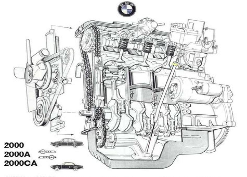
1966 - 1972 100 bhp @ 5500 rpm 157 Nm @ 3000 rpm
