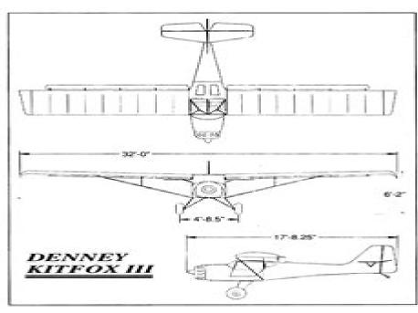
About the only enursal design feature of the Kittux is the detached alterons, which are entirely separate serfaces suspended just below the trailing edge of the wisq (see three-view). The model pictured was built from Clave's plans and photographed by Git Caughtin of Tacona, Washington.
