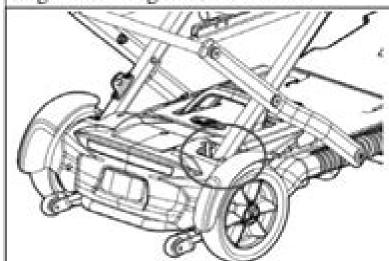
Make sure the free-wheel lever is in the engaged position
