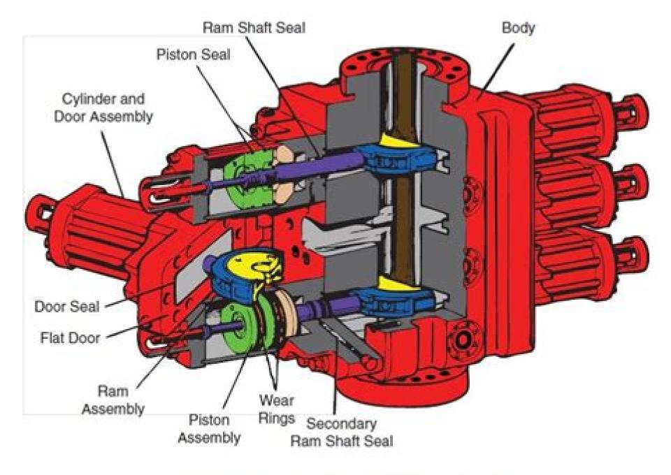
Figure 2-1. Manual Lock SL Blowout Preventer
