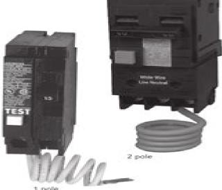
Siemens GFCI circuit breakers are UL Listed and CSA. Certified as Class A devices, Current imbalances of 4-6 milliamos or more between load conductors will cause the ground fault sensor to trip the circuit biographies.
