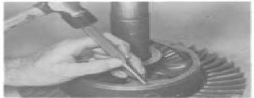
Use a hammer and center punch to secure the groove pins. This will prevent the groove pins from moving.
