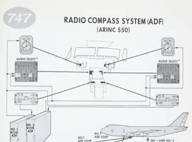
AUDIO SELECT PANELS ARE ALSO LOCATED AT THE ENGINEER'S STATION. AT THE PIEST OBSERVER'S STATION SECOND OBSERVER, OPTIONALL AND AT THE MAIN EQUIPMENT CENTER.
