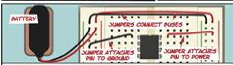
YOU CAN MAKE CONNECTIONS BETWEEN ROWS OF TIE-POINTS BY INSERTING SHORT PIECES OF WIRE CALLED JUMPERS BETWEEN HOLES IN DIEEPPRIT DOWN.
