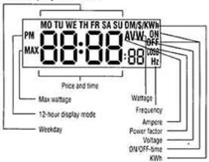
The PM 230 electricity meter is a monitoring and testing instrument with which it is possible to determine the power consumption of a connected appliance and the cost of the electricity consumed.
