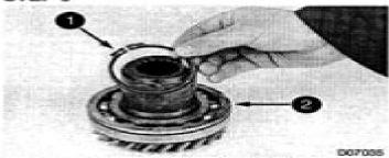
Remove the snap ring (1) from the coupling shaft and remove the bearing.
