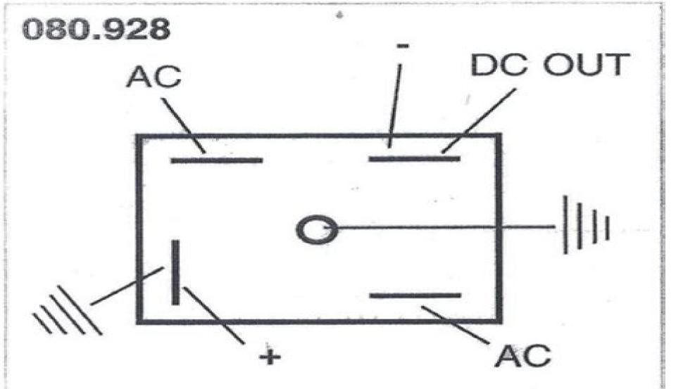
Wiring diagram shows positive earth system for negative earth reverse polarity (Neg to earth pos to DC out) on three lead stators bridge 2 leads in one AC in
