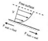
Flow of an unconfined viscous fluid down an incline.
