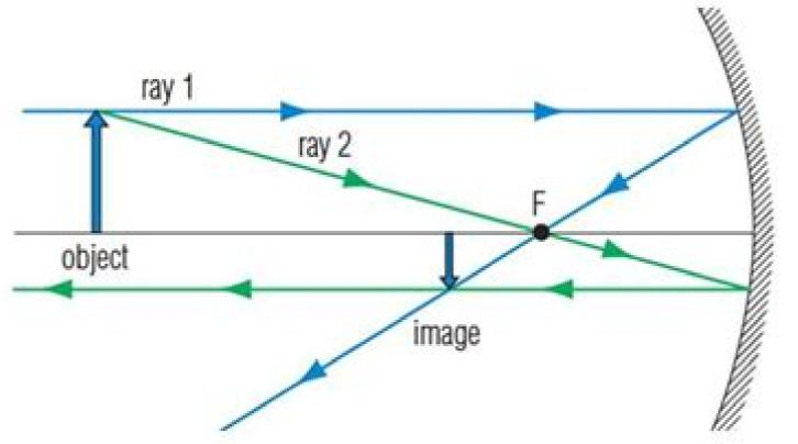
Ray 1 - travels parallel to the principal axis and reflects through the focal point (F)
