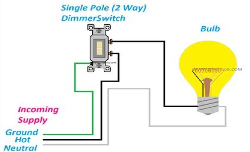
Single Pole(2 Way) Dimmer Switch Wiring Diagram
