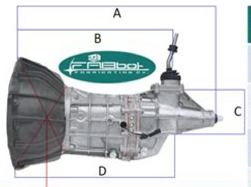
Picture not representative of transmission with FABbotFab Bellhousing or adapter plate installed, dimensions are representative
