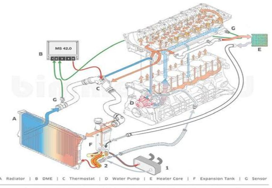
1 Transmission Heat Exchanger | 2 Heat Exchanger Fittings on Expansion Tank (to radiator)
