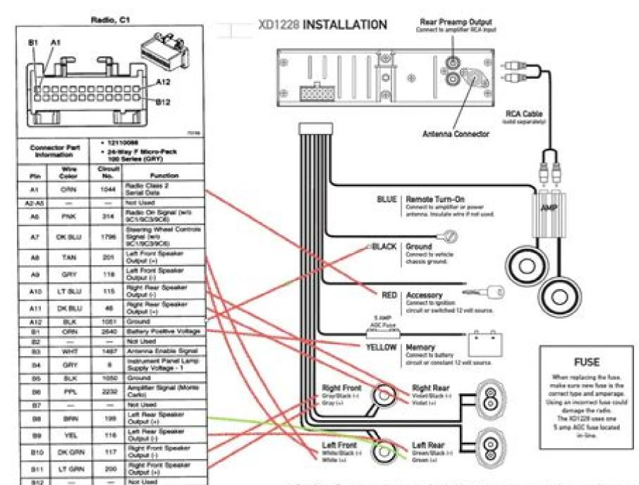
" Caution - Do not attach any speaker leads to ground as severe damage will occur.
