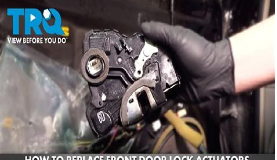
HOW TO REPLACE FRONT DOOR LOCK ACTUATORS 2007-2011 TOYOTA CAMRY
