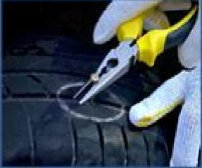
Step 2 Remove the object caused the puncturewith plier
