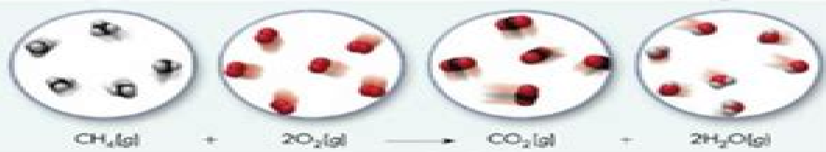
Figure 20.1 Oxidation of Methane In a Bunsen burner, oxygen from the air is mixed with methane from the gas line. The methane is oxidized, and carbon dioxide and water are produced.
