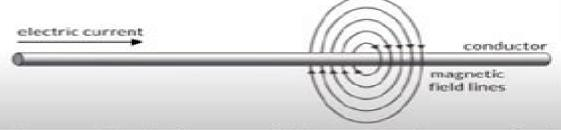
When you uncoil a solenoid, you essentially have a straight wire. A current flowing through this wire generated a magnetic field around it, but this field is relatively weak and spread out.
