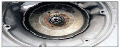
As with other thrust washers, lightly grease both sides to hold them in place and place the tabs in the three recesses or holes of the sun gear shell.
