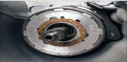
To be sure that it stays on, lightly grease both sides of the thrust washer and install in on the rear planeters.
