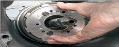
Lubricate the individual pinion gears with transmission fluid or special assembly fluid; grease the gear teeth and the wear surface on the planetary body and "rotate" it into the rear annulus gear. It fits almost even with the low-reverse drum's outer flange.
