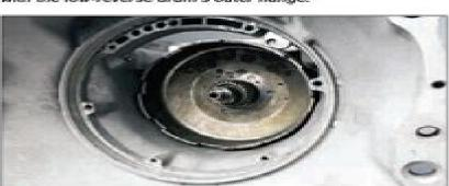
Lubricate the inner bushings and teeth of the sun gear and grease the steel thrust plate. Rotate and slide it onto the output shaft.
