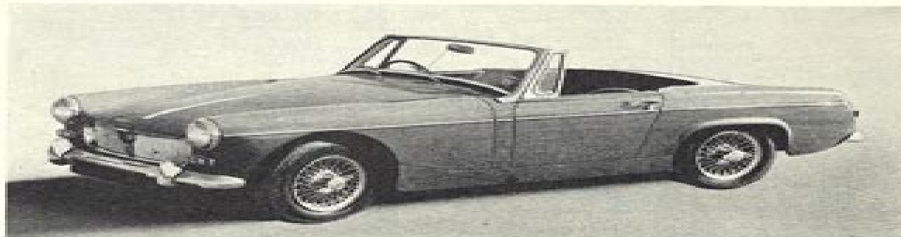
DISTINGUISHING FEATURES: Swivelling quarter lights and wind-up windows identify the Mark II cars in latest form, although styling in general follows the lines of previous models.
