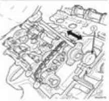
Fig. 37 Consthalt End Play Measuring: \$10 Date to the contract of th
