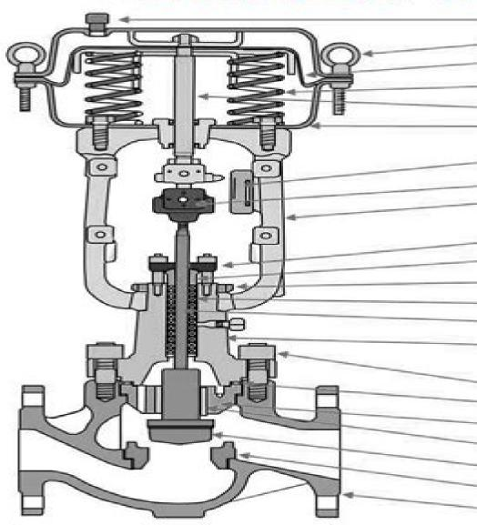
Rain cap Eye bolt Diaphragm Spring Actuator stem Diaphragm case
