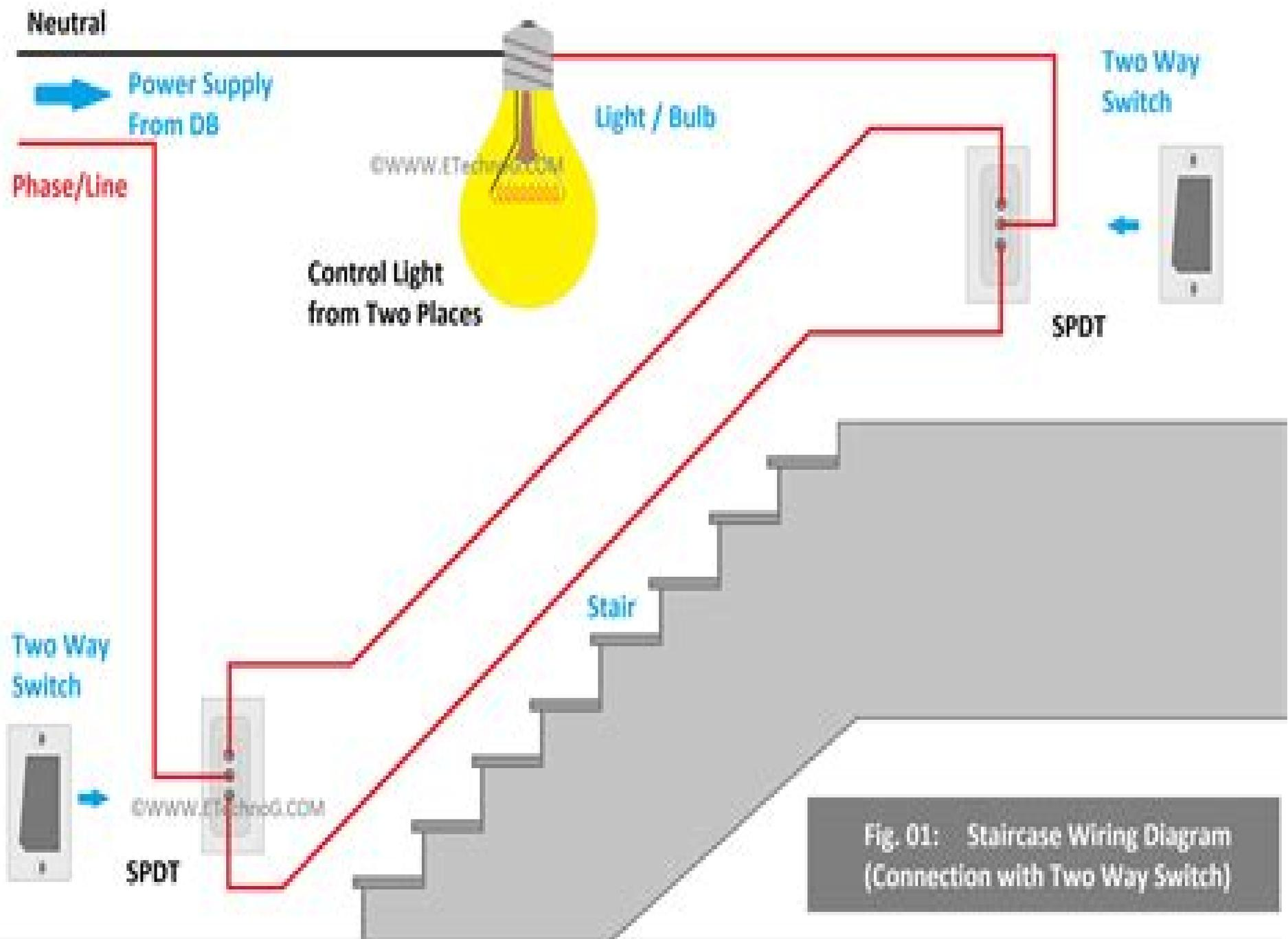
Fig. 01: Staircase Wiring Diagram (Connection with Two Way Switch)
