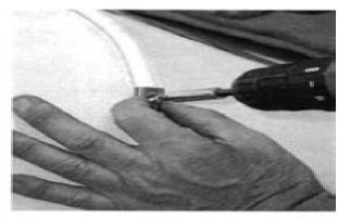
28 The final step is to install the new wire-on strip that comes with the new canvas. It's first stapled into place with long staples, then trimmed to size. Next, it's folded in half and tapped down with a hammer before the ends are screwed into place, as shown.
