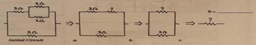
The circuit below is similar to Figure 35-11 in your textbook. In three successive steps, as in Question 1, replace each pair of resistors by a single resistor of equivalent resistance.
