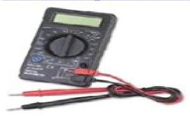
The DT830B digital multimeter is a compact, light tool - a bargain if you need something cheap and reliable. The heart of the instrument is the ICL7106 IC coupled with a large 3 1/2 digit, 7 segment, 0.5" high LCD display with a maximum reading of 1999.
