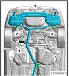
Stress-free alignment of exhaust system 1.4
