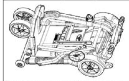
Pull the red lever on the side of the scooter and begin unfolding it from the tiller.
