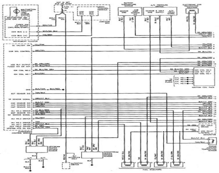
Engine control system - 1995 and 1996 four-cylinder models (1 of 4)
