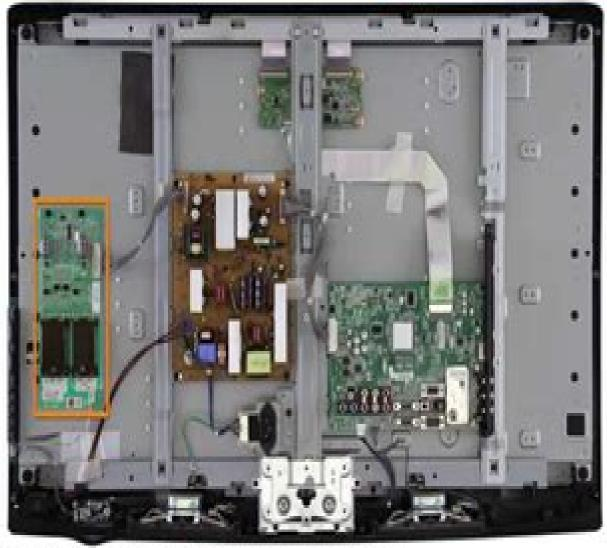
Locate Backlight Inverter Board
