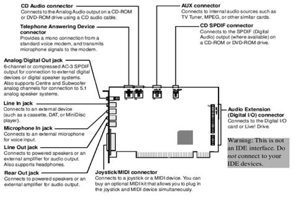
Figure 1-1: Jacks and connectors on the Sound Blaster Live! card.
