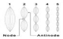
The wavelength of a standing wave can be found by measuring the length of two of the "bumps" on the string. The first harmonic only contains one bump, so the wavelength is twice the length of the individual bump.
