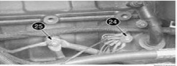
Remove nut (24) and washer from engine ground stud. Disconnect secondary steering ground wire (if equipped) and five ground wires of the rear chassis wiring harness from stud. Remove nut (25) and washer. Disconnect ground cables from engine ground stud. Move cables away from engine.
