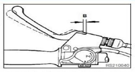
Set to distance B at the handlebar lever by turning adjusting screw (2) on the clutch release lever.
